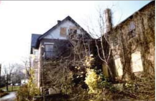
Boarding up without adequate ventilation and maintenance has accelerated deterioration of this property. Photo: NPS files.
