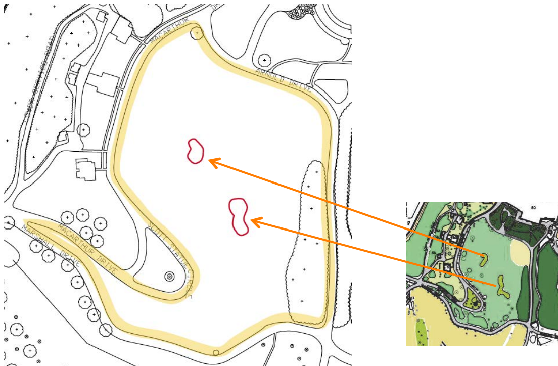
Figure 21: The two Contributing evergreen clusters will be protected by temporary construction fencing as shown on this plan.
