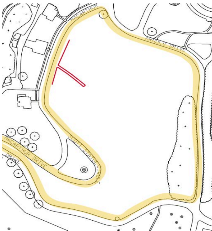
Figure 26: Known aboveground and belowground remnants of historic pathways will be protected by temporary construction fencing, as shown on this plan.
