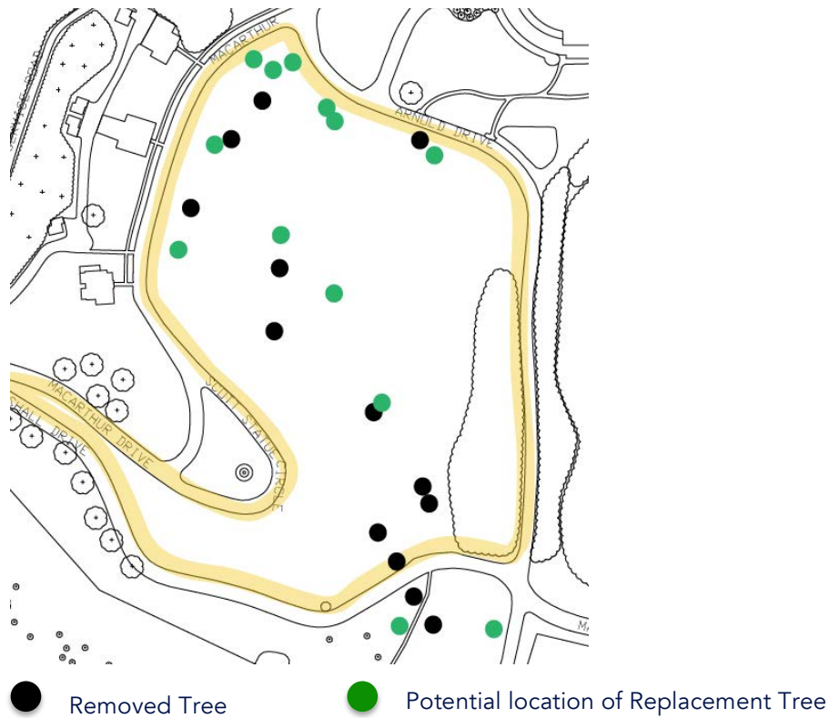
Figure 27: Plan of trees proposed for removal and concept for locations of replacement trees. New tree locations are based on general location of removed trees and/or 1914 tree locations where possible.
